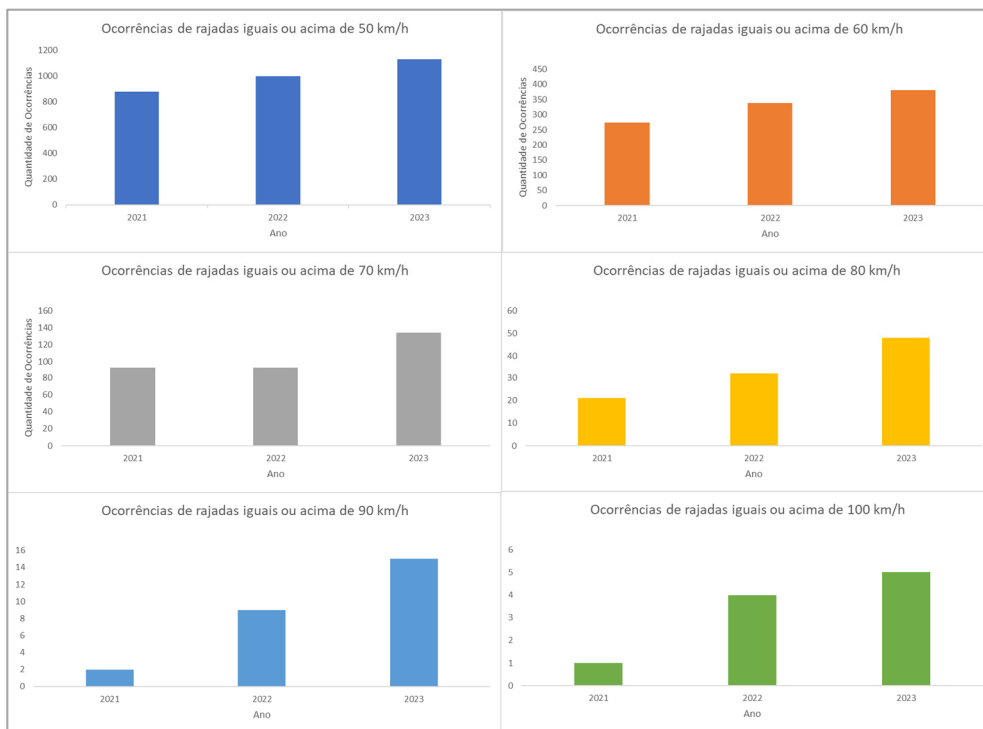
Figure 4 – Number of occurrences for different maximum daily gust values. Source: Adapted by Cemig from data of INMET.
